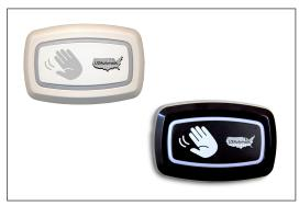
The push-to-operate wireless button operates at 433.92 MHz in AM/ASK modulation.
